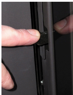
Im. 3: Opening the door left side for cleaning
